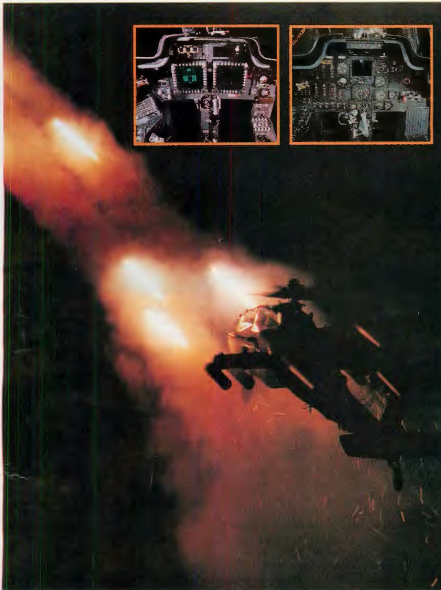
AH-64D Longbow Apache fires 70mm CRV7 air-to-ground rockets during tests at Army's Yuma, Ariz., Proving Ground. A born hunter, nothing is safe on ground or in the air when Longbow Apache is on prowl. The AH-64D Longbow Apache pilot's crewstation (left inset) is a leading-edge installation, even compared to the state-of the art AH-64A version. (below) AH-64D Longbow Apache is equipped with mast-mounted Longbow Fire Control Radar, key to its mastery of the battlefield.
